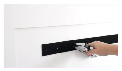
Once the buttons are all on, add heavy duty velcro to the back of the headboard using the staple gun.
