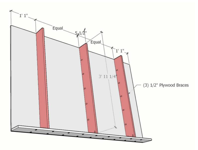
Drill pocket holes in the 3 plywood center slats approximately 8 inches apart. Add the center slats to the large piece of plywood using pocket screws and wood glue.
