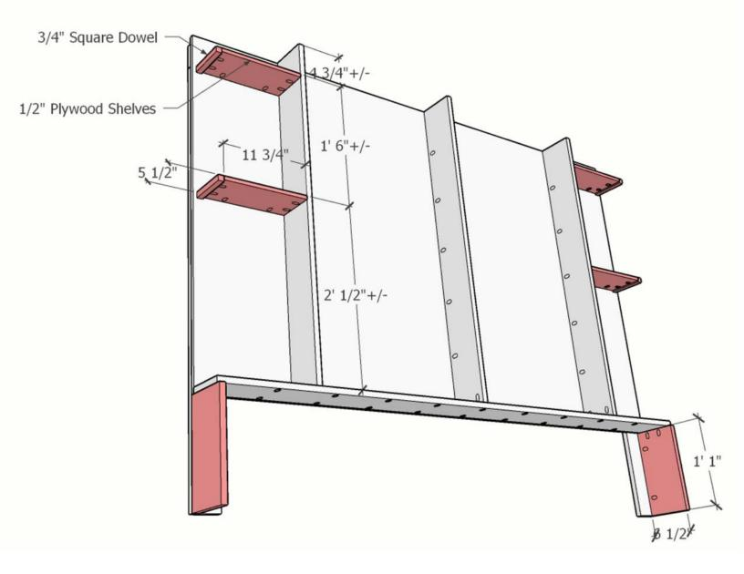
I chose to add 2 shelves, but you can add as many shelves as you would like. To finish off the edge of the plywood shelf, add the square dowel to the edge with either brad nails or pocket holes. You could also use veneer banding. Attach both the shelves, and the leg pieces, using pocket holes and pocket screws.
