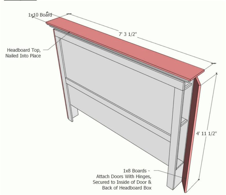
Nail the 1x10 board on the top to finish it off. Now all you need to do is add the doors using two 3" basic hinges. The door is cut to be slightly shorter than the legs to prevent any dragging on the carpet.
