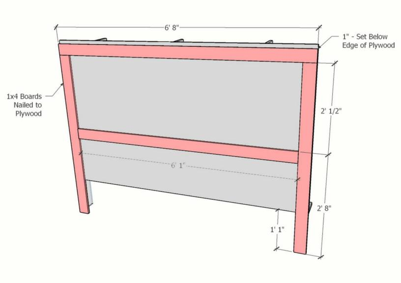
On the reverse side of the plywood, add the 1x4 pieces using wood glue and brad nails. Leave 1 inch of space at the top of the plywood for the crown molding to be attached to in a later step. If you don't want to add a tufted insert, you could add 2 additional vertical 1x4 boards to create a grid pattern.
