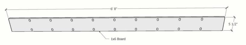
Using a drill and the pocket hole jig, drill pocket holes approximately 8 inches apart. This 1x6 board will be come the bottom of the headboard.
