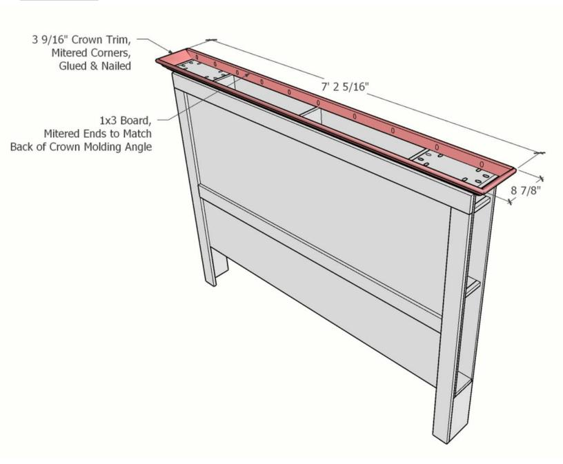
It's time to add the crown molding! Atach it to the front and the sides using a brad nailer and wood glue. The back of the headboard needs to be flat so it can be up against the wall, so you will not be using crown there, but will instead add a 1x3 board. The ends will need to be cut at an angle so they align with the edges of the crown molding. This piece gets added using pocket holes and pocket screws.
