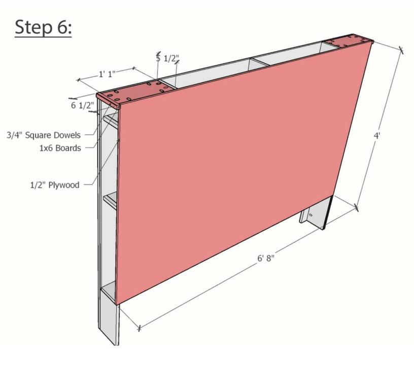
The second piece of plywood is now added to become the back of the headboard. Use wood glue and screws to attach it to the bottom as well as the center slats. Drilling a pilot hole before adding the screws helps the plywood not to split. To create a top for the shelves, add the 1x6 pieces using pocket holes and pocket screws. The square dowel on the end of it will stick out past the edge of the headboard. This is to account for the thickness of the doors.
