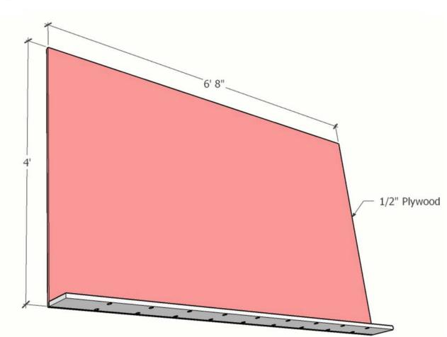
Attach the 1x6 to one of the pieces of plywood using pocket screws and wood glue. The pocket screws should be facing down.
